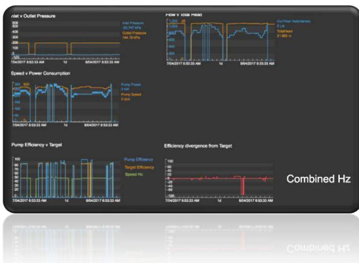
The 'raw' operational data together with analysis results are presented in a dashboard allowing users to see current performance, performance at different speeds, and performance over time at a glance.
